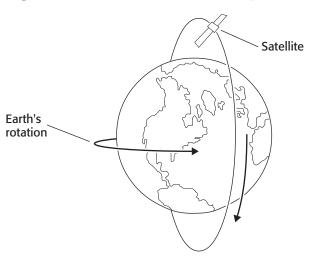
Weather satellites in polar LEO can provide detailed information about the weather in an area.
