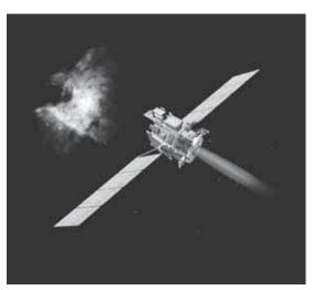
Deep Space 1 uses an ion rocket to move.
