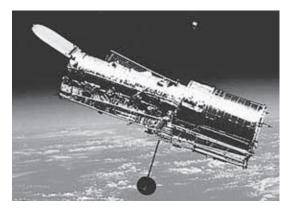
The mirrors in the Hubble Space Telescope are smaller than the mirrors in many telescopes on the Earth. However, the Hubble Telescope can produce images of very faint objects because the Earth's atmosphere does not blur the images.
