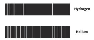
These are the emission spectra for the elements hydrogen and helium. These two elements make up most stars. Each line represents a different color of visible light.
