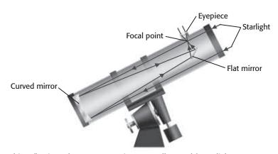
This reflecting telescope uses mirrors to collect and focus light.
