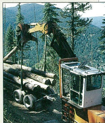
Logs are loaded onto a truck for their trip to a sawmill.
