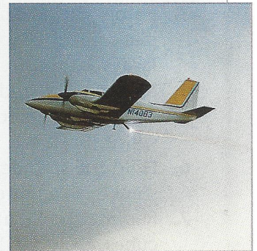
An airplane drops crystals of silver iodide to try to make rain.
