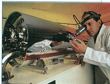
This atomic clock is from the National Institute of Standards and Technology. The long cylinder is the clock.
