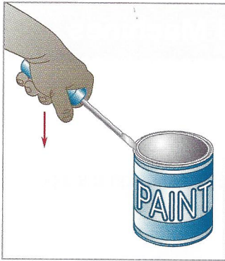
Figure 17-3 This screwdriver is being used as a lever.
